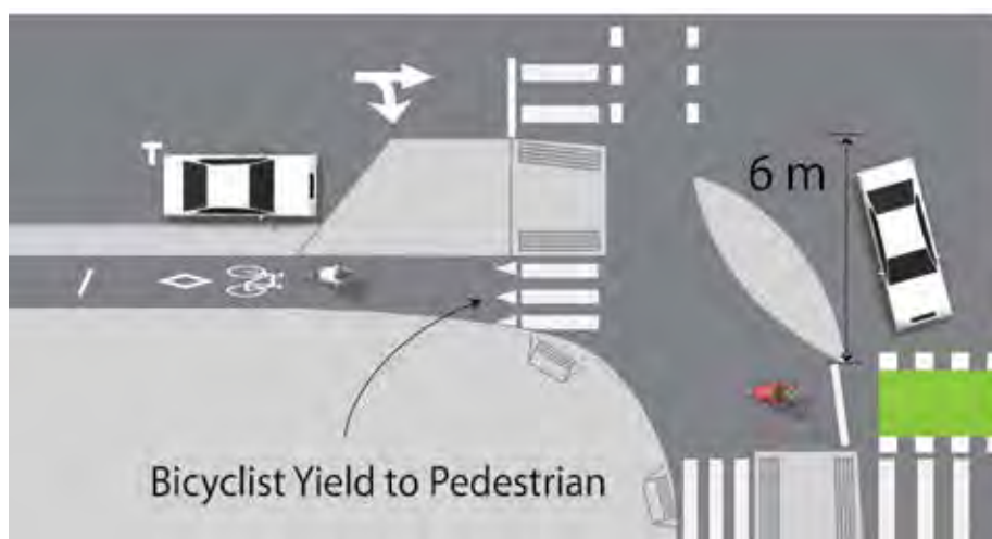
Figure D.2: Cycle Track at a Corner Refuge Island
