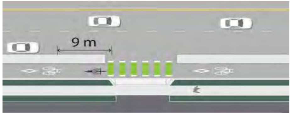
Figure D.10: Driveway Crossing Retrofit
