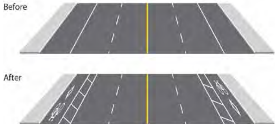
Figure D.15: Roadway Widening to Create Pedestrian and Bicycle Accessible Shoulders
