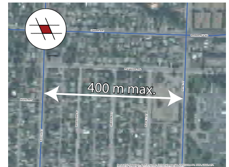
Figure 3.1: Mesh width standard - Core Area
