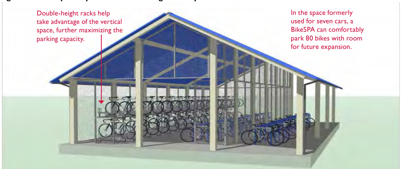
Figure 6.17: Sample Bicycle Secured Parking Area layout
