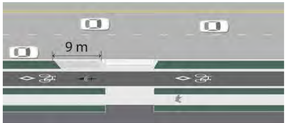
Figure D.11: Driveway Crossing Reconstruction
