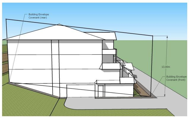
Diagram 13.9: 13m Maximum Height As Measured From Straight Line Between Building Envelope Points
