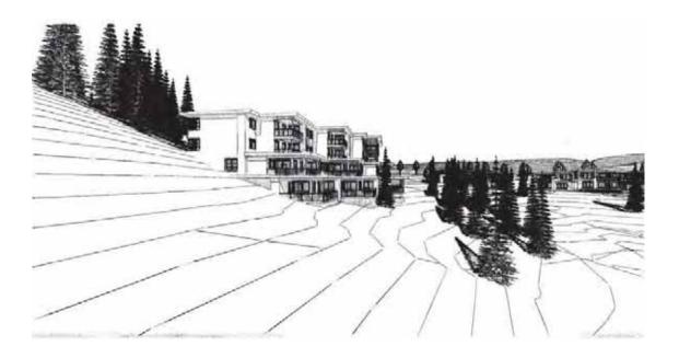
This site has a general slope of less than 4:1, allowing for construction of the proposed building without the need for extensive retention works and allowing for the retention of natural grade
