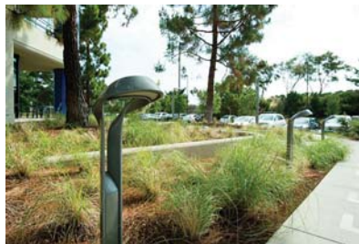
BOLLARD LIGHT: Model: Metro 40 Lo Glo Height: 914mm Colour: Powdercoat Silver Manufacturer: Landscape Forms www.landscapeforms.com
