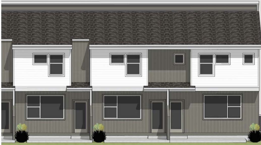
East/West Elevation Detail showing breaks in vertical & horizontal planes. Materials accentuate the breaks and provide additional human scale
