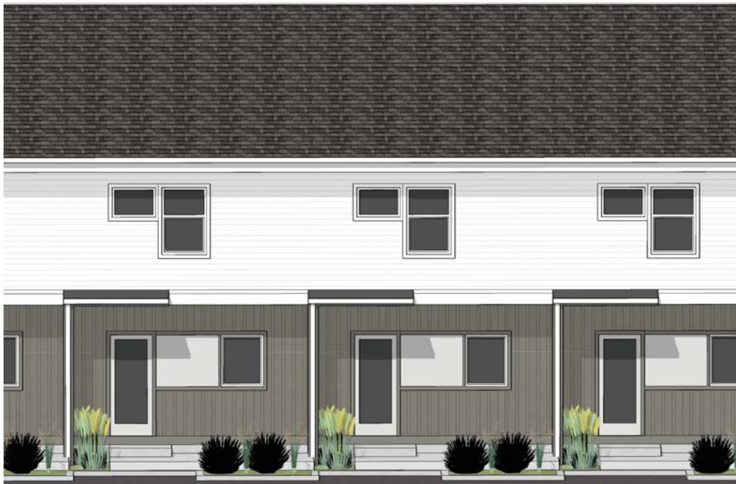
Interior (parking plaza) elevation detail showing breaks in vertical & horizontal planes. Materials accentuate the breaks and provide additional human scale
