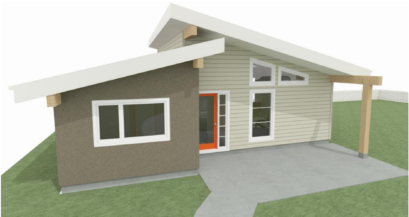
Figure 1. Elevation of proposed carriage house.
