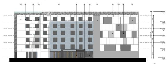
The south portion of the building, facing the highway, will not have windows. It is intended that the second building tie into the first during the second phase of construction. To avoid the possibility of a blank portion of wall façade, the building will be clad in a variety of panel colours, providing a degree of visual interest during the building phasing.
