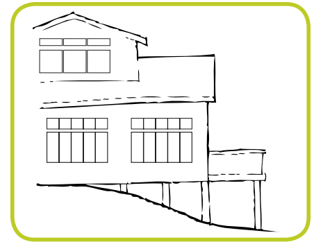
4.0 - Example of house with deck not well integrated with the hillside
