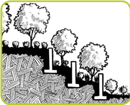
3.0 - Terrace retaining walls to reduce cut and fill and minimize height
