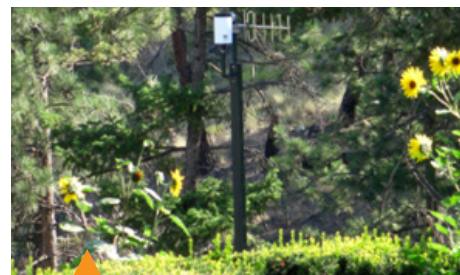
Data on stormwater is collected through automated rain gauges located throughout the City. There is over 30 years of historical data available.
