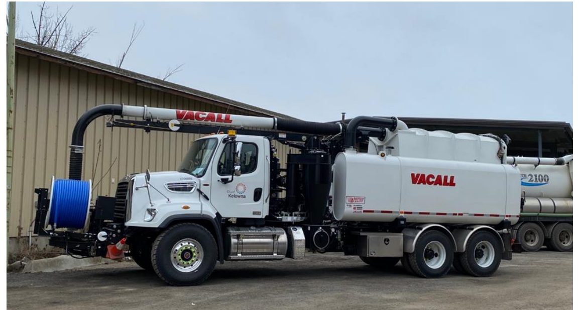
Vac-Truck used to regularly to clean out Catch Basins and drains
