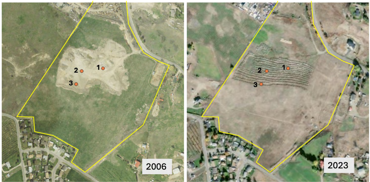
Figure 3. Aerial photographs showing the extent of the gravel excavations (2006) and current location of fill placement (2023). Soil pits examined and described in this report are shown as numbered points.
