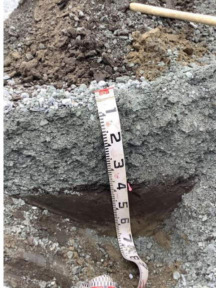
Figure 6. Depth of crush gravel present on one portion of the gravel parking area
