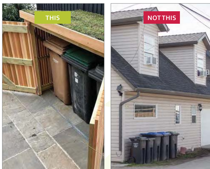
Figure 36: Ensure that site layouts include provision for solid waste pick-up and bin storage that is enclosed or otherwise screened from view (3.3.4. b).
