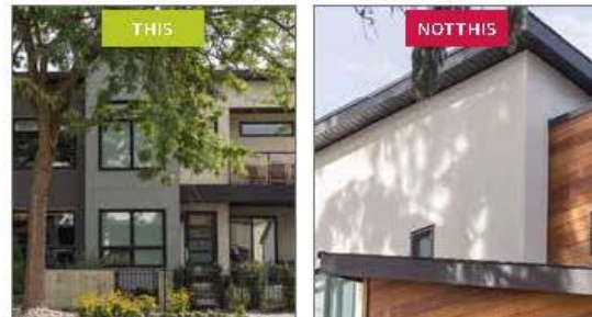
Figure 28: Front doors should be directly accessible via a walkway, porch and/or stoop, and front yards should incorporate complementary landscaping and modest fencing (3.3.3 c, d).
