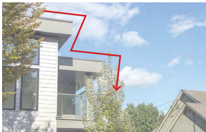
Figure 31: Use building height, scale and setbacks to limit height differences between new and existing development in the surrounding area (3.3.2 c).
