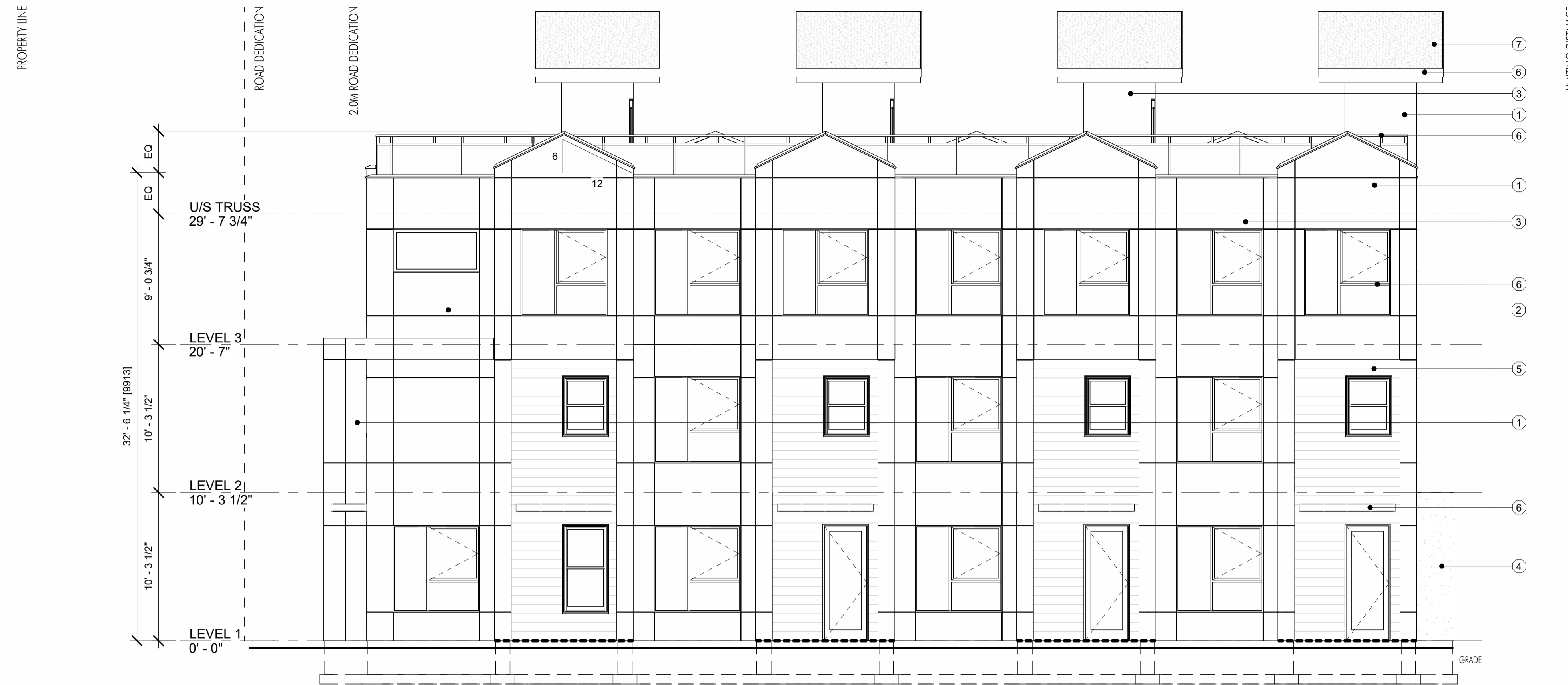
1 BUILDING 1 - SOUTH ELEVATION A-202 3/16" = 1'-0"
