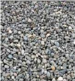
ROOFING MATERIAL GRAVEL BALLAST
