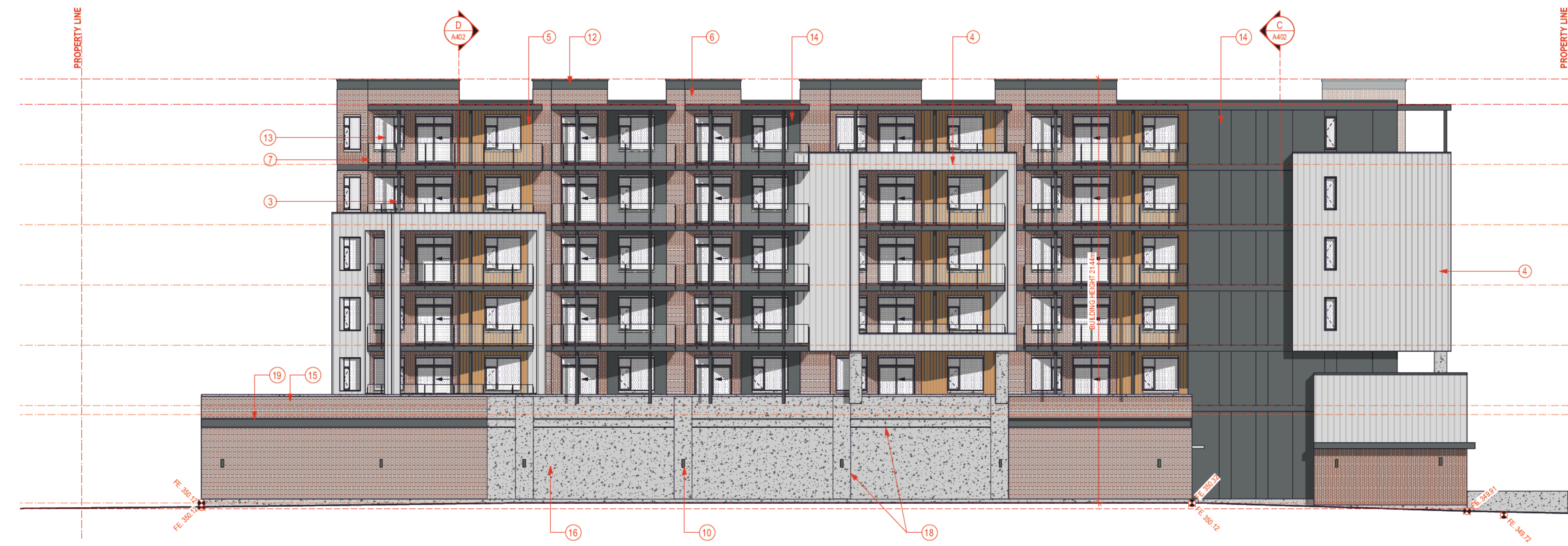
2 BUILDING ELEVATION - NORTH Scale: 1:120
