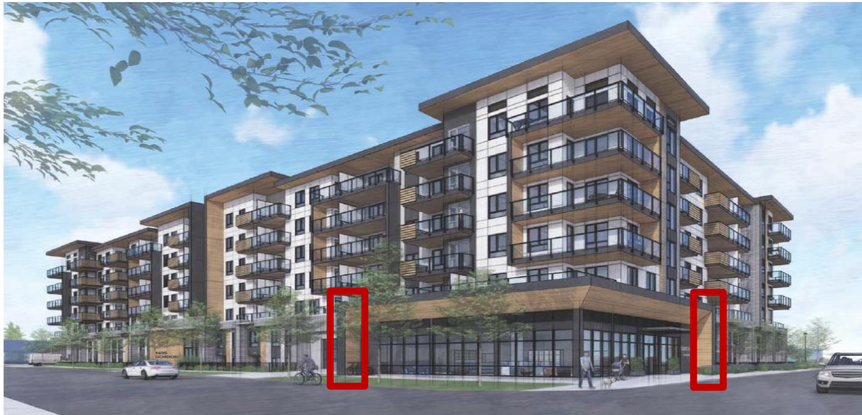
Fig 1: Setback variances shown in red for structural columns supporting roof canopy above the daycare.
