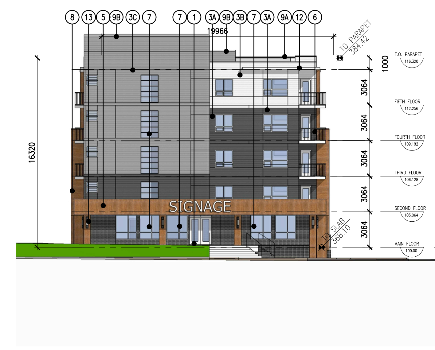
BUILDING 1 EAST ELEVATION SCALE: 1:200
