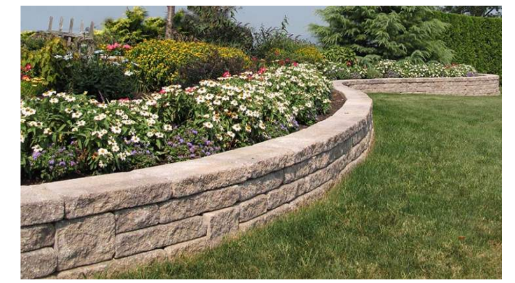
PRECAST BLOCK PLANTER Allan Block Splitfaced Planters On Slab (or Approved Equivalent)
