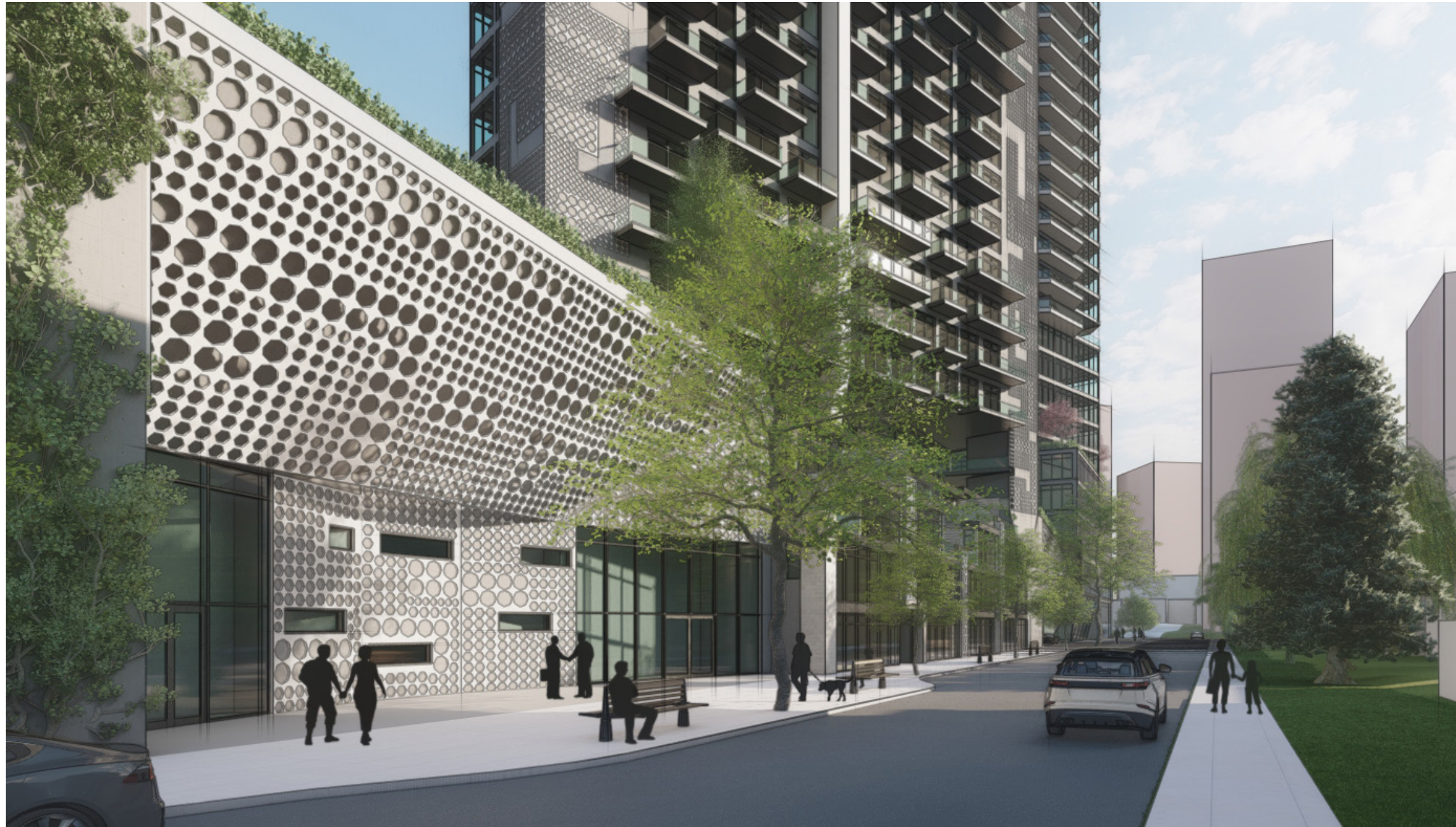
Perforated architectural screen concealing above-grade parking structure.
