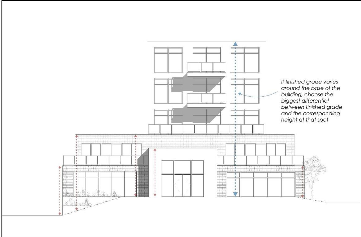
Figure 5.3(c) – Finished Grade: Sloped Fronting Road
