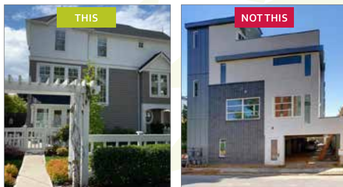
Figure 18: In 'shotgun' townhouse projects, ensure that the end unit facing the street is a true street-oriented unit (3.1.1 d).
