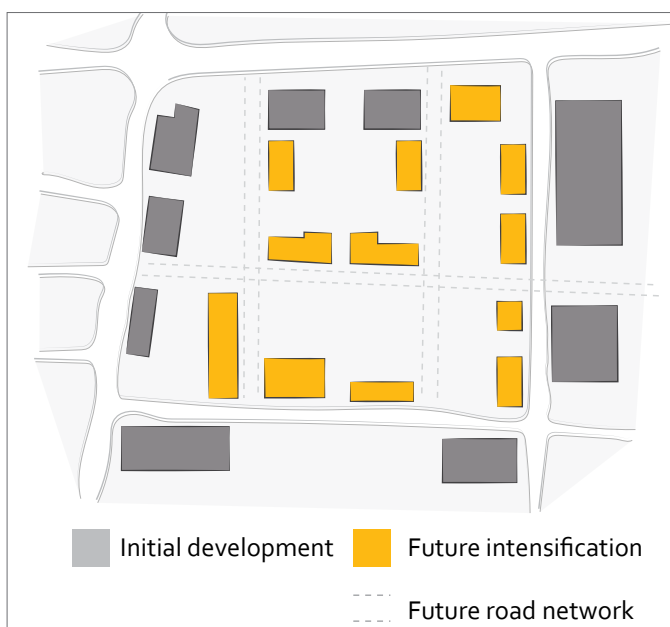
Figure 65: Base new retail, commercial and industrial development on an internal circulation pattern that can easily accommodate redevelopment and future intensification (6.1.2 i).
