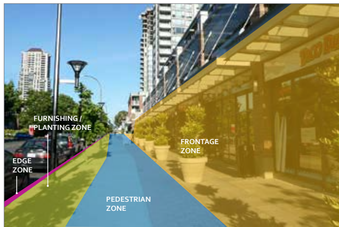
Figure 45: The sidewalk interface can be broken down into four zones, all of which have a role in supporting walkability, social interaction, and strong retail accessibility and visibility (5.1.1. g).
