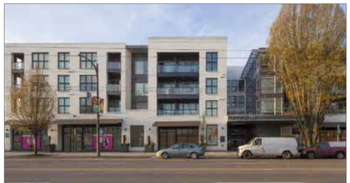
Figure 39: An example of breaking down a long building facade, using recesses to articulate the facade and allow shadows to add detail and variety (4.1.6 a).
