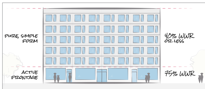
Figure 14: While retaining at-grade transparency, targeting lower window-to-wall ratios on building elevations can significantly reduce energy demand. As general guidance, designers targeting the Lower Steps of the Step Code should target no more than a 50% WWR and designers targeting the Upper Steps should target a WWR of less than 40% (2.2.1 c).
