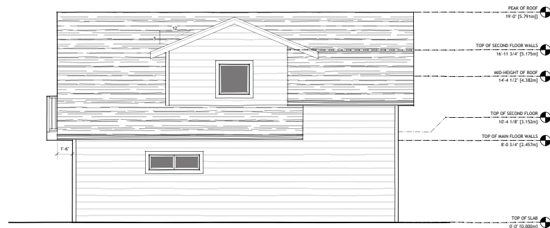
3 CARRIAGE HOUSE SOUTH ELEVATION Scale: 1/4" = 1'-0"
