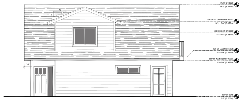
1 CARRIAGE HOUSE NORTH ELEVATION Scale: 1/4" = 1'-0"
