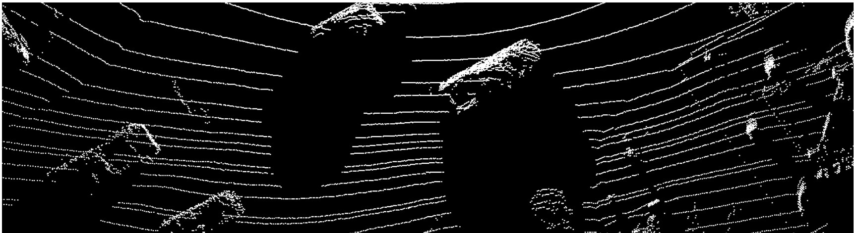
Figure 6 The figure above depicts the output of a LIDAR sensor installed in downtown Kelowna. LIDAR technology, which works similarly to radar, powers most self-driving vehicles. Within the Central Okanagan, LIDAR is currently being used in flood mapping and transportation studies among other applications.
