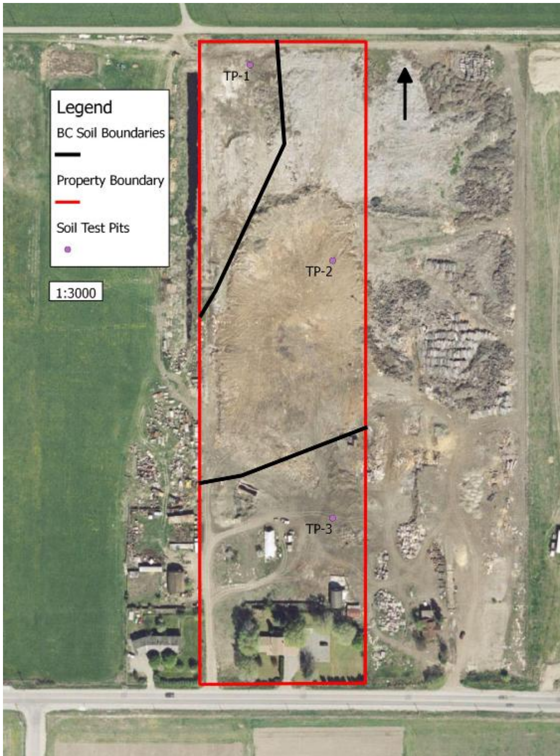
Figure 9: 982 Old Vernon Rd. Kelowna BC – Soil Inspection, Soil test pit location map
