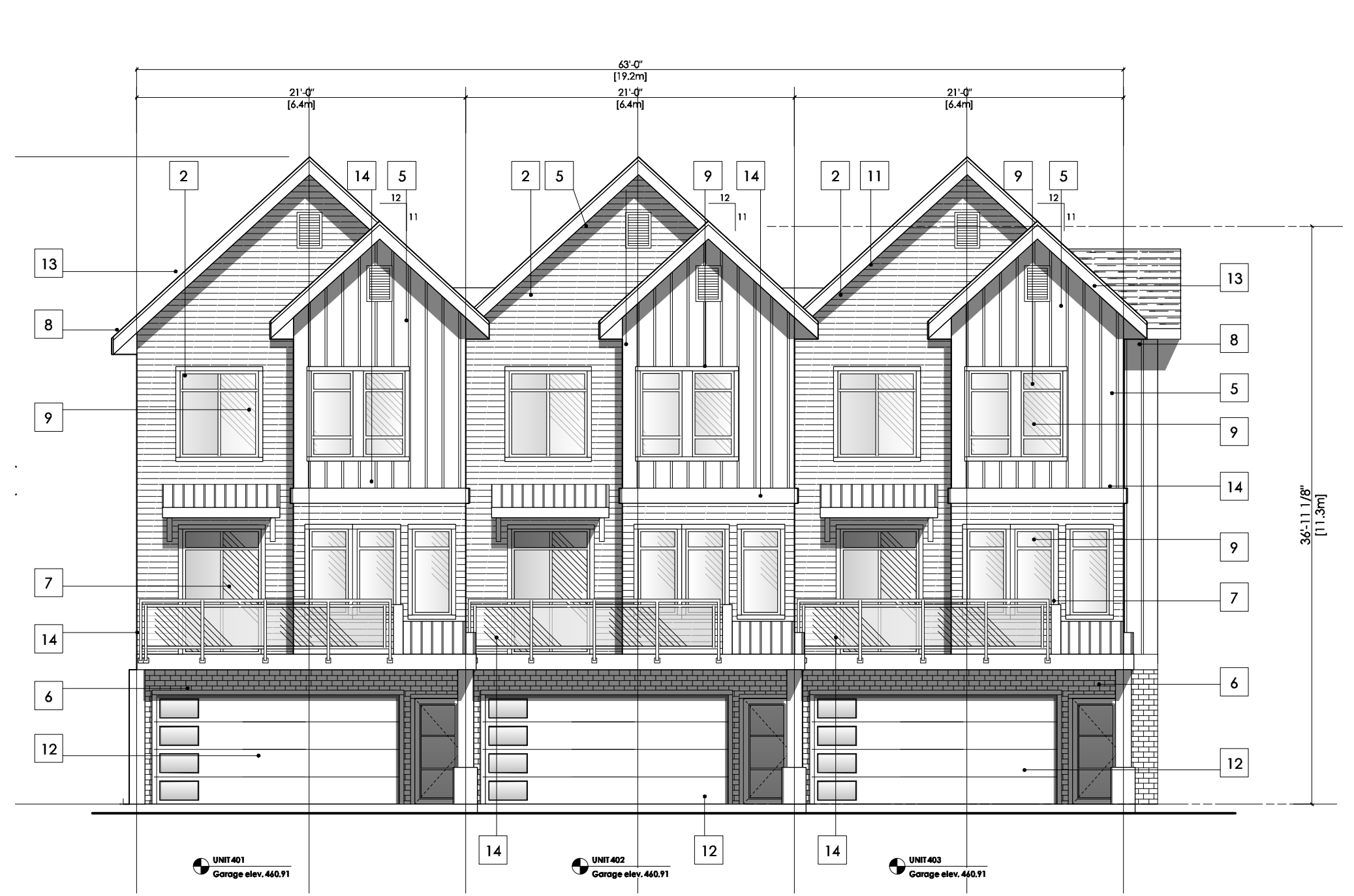
E-1 Building 4 - Lane Elevation Scale 1/8" = 1'-0"
