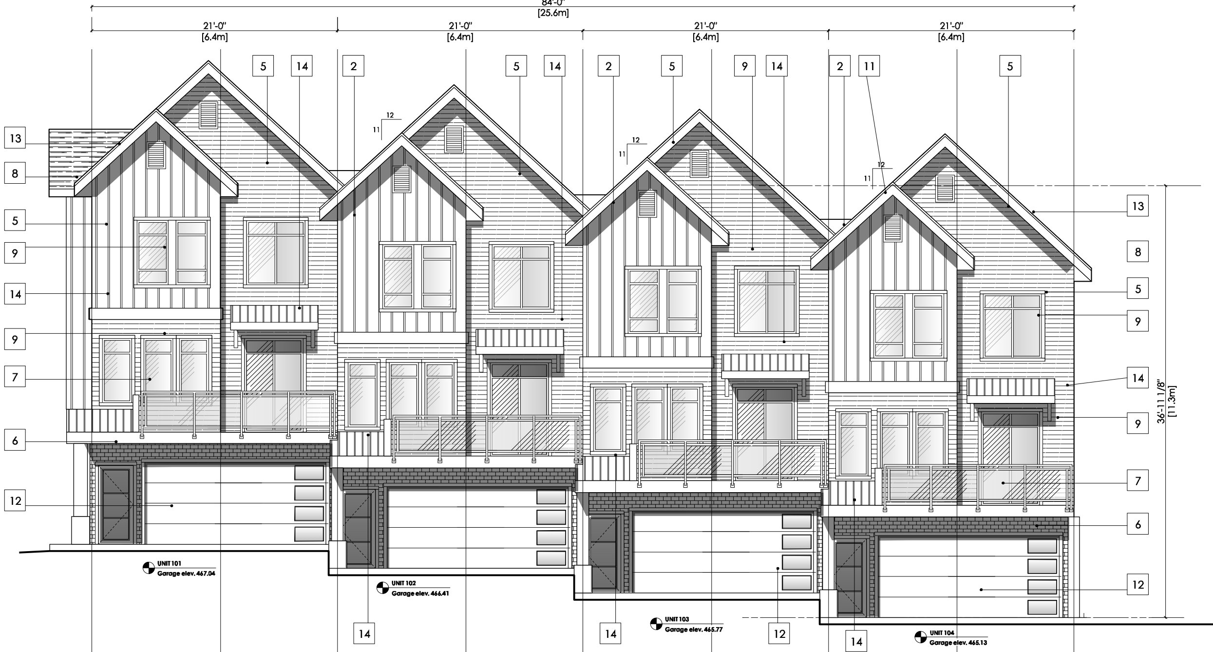
E-1 Building 1 - Lane Elevation Scale 1/8" = 1'-0"
