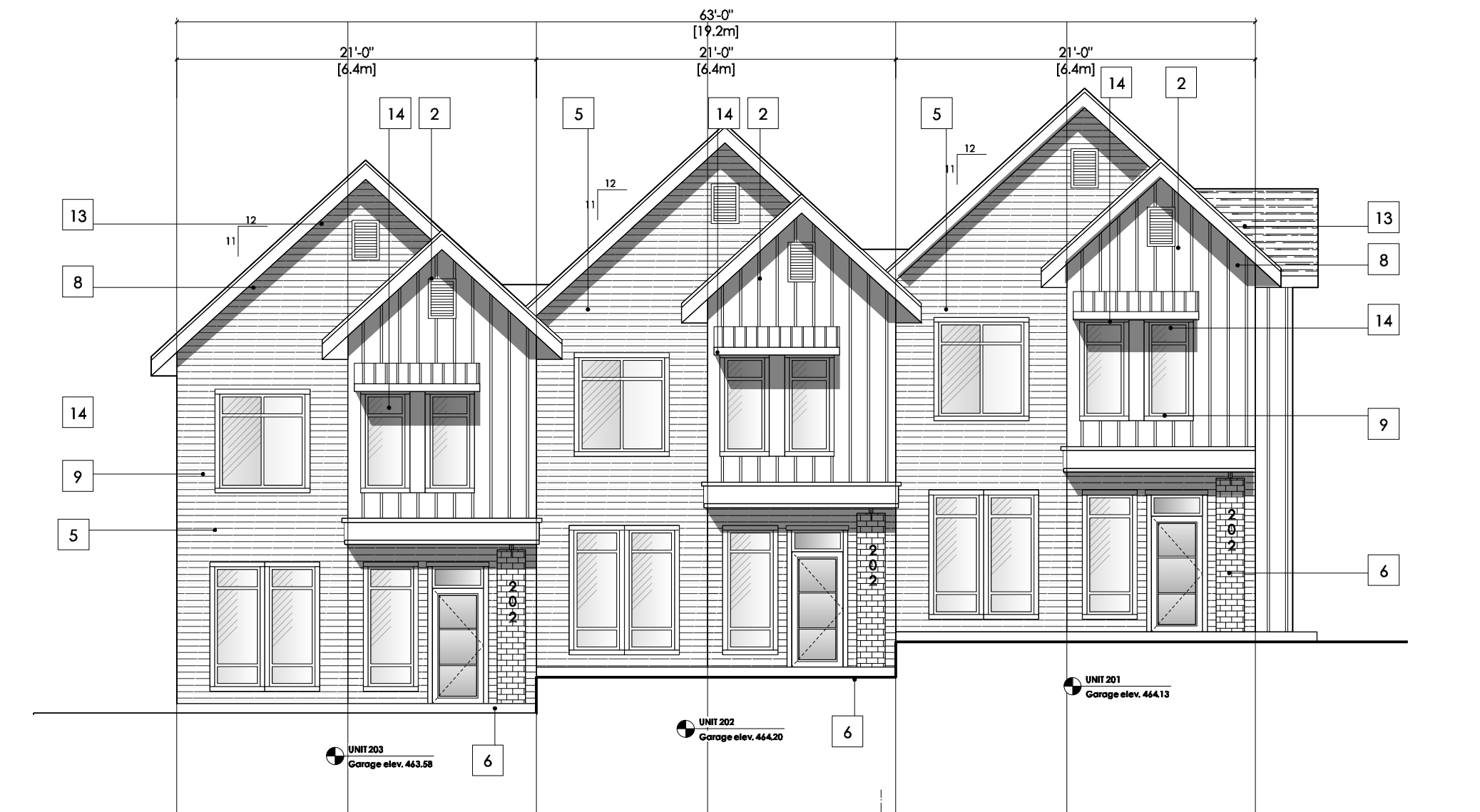
E-2 Building 2 - Clifton Elevation Scale 1/8" = 1'-0"
