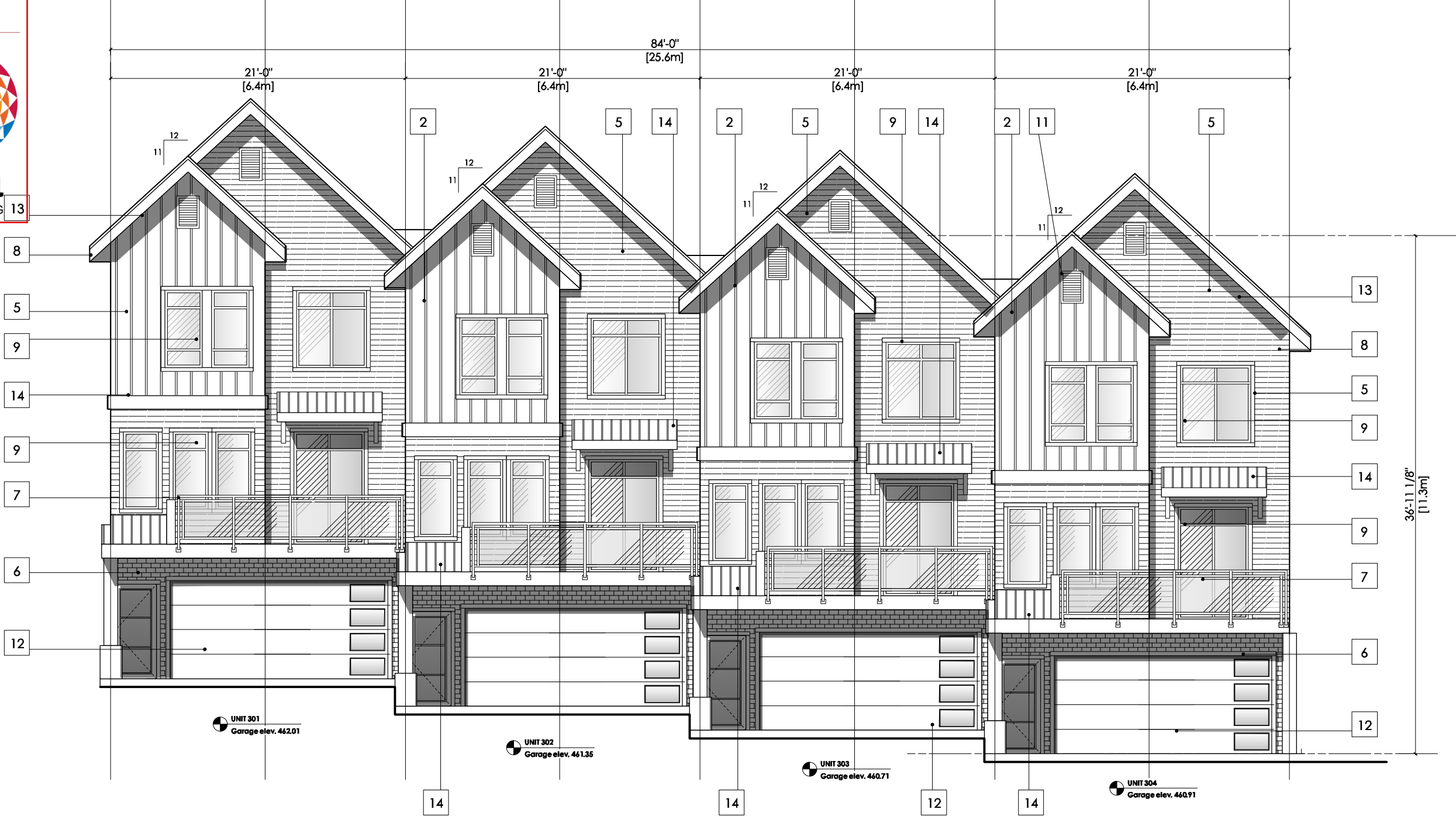
E-1 Building 3 - Lane Elevation Scale 1/8" = 1'-0"
