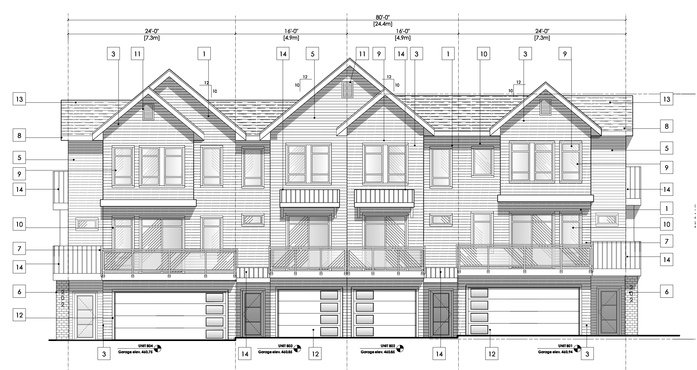
E-1 Building 8 - Lane Elevation Scale 1/8" = 1'-0"
