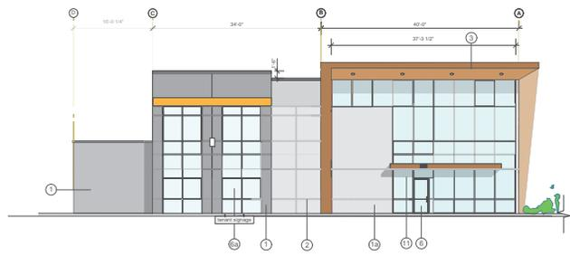
11 West Elevation - Pier Mac Way Elevation for Glazing Calculations
