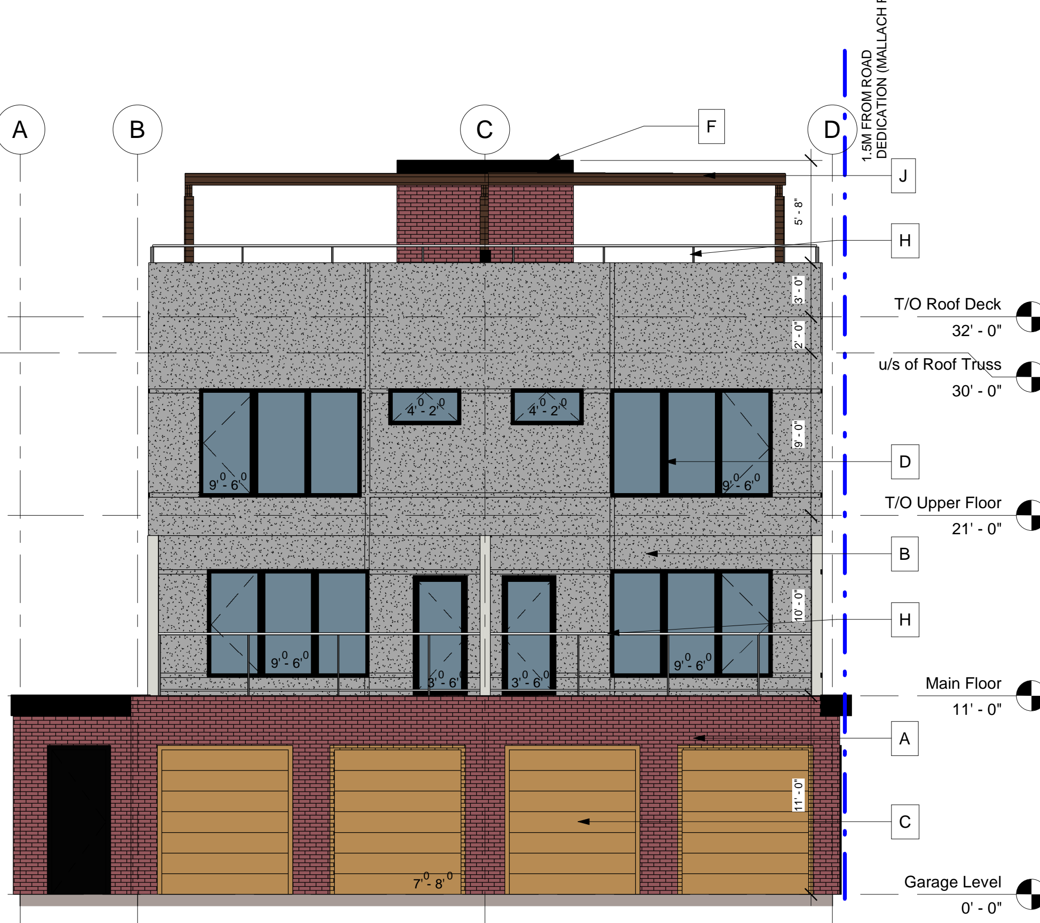
BLDG 1 -East Elevation (Mallach Rd.) 3/16" = 1'-0"
