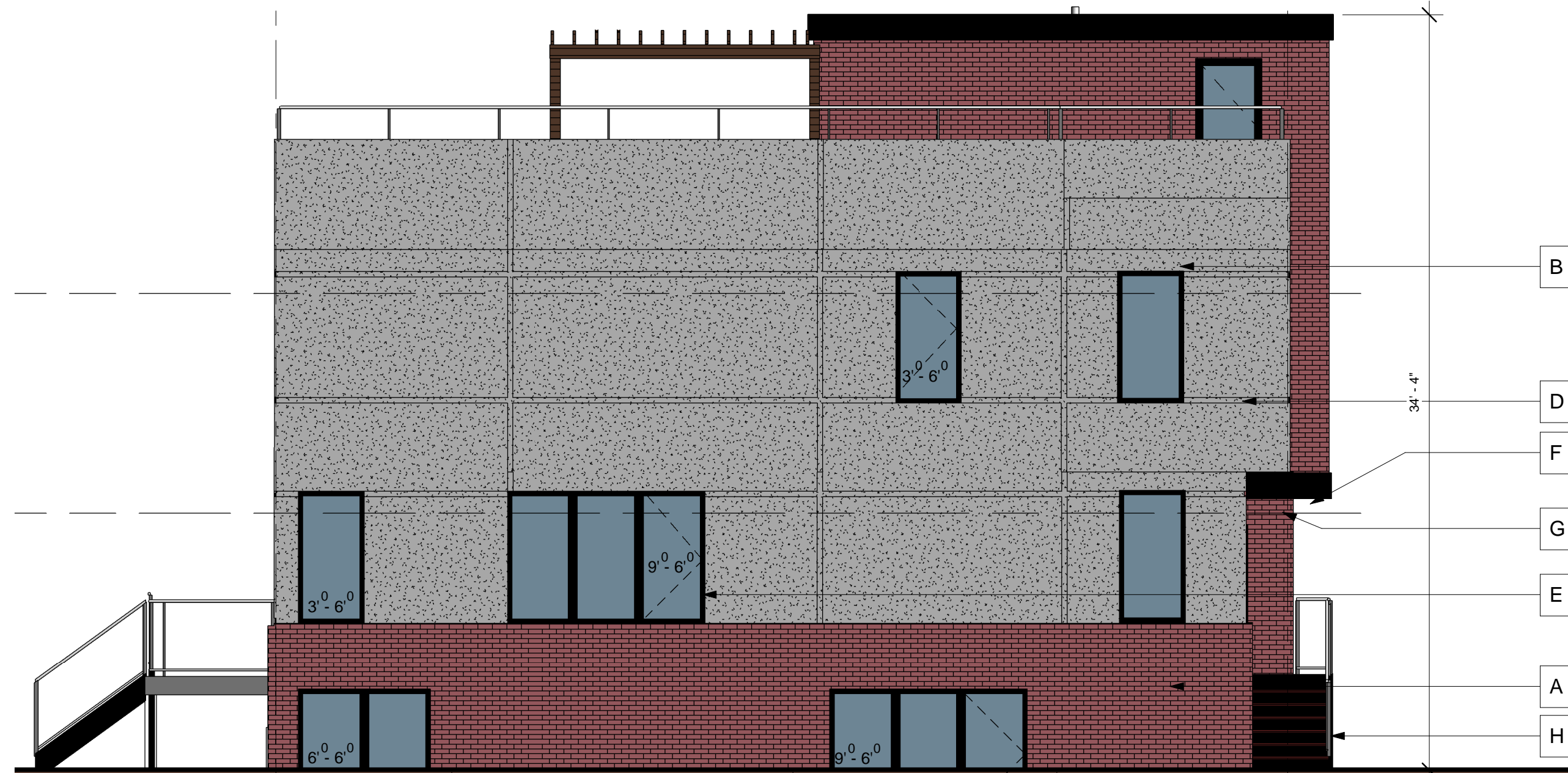
1 East Elevation-BLDG 2 (Mallach Rd.) 3/16" = 1'-0"
