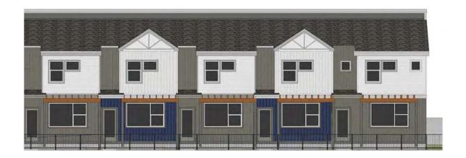
East/West Elevation Detail showing breaks in vertical & horizontal planes. Materials accentuate the breaks and provide additional human scale
