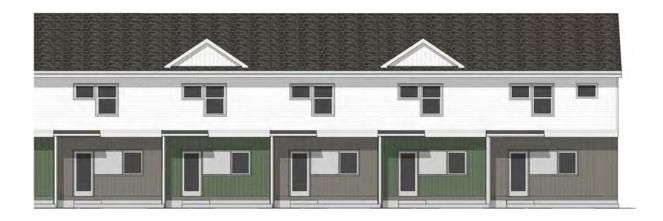
Interior (parking plaza) elevation detail showing breaks in vertical & horizontal planes. Materials accentuate the breaks and provide additional human scale
