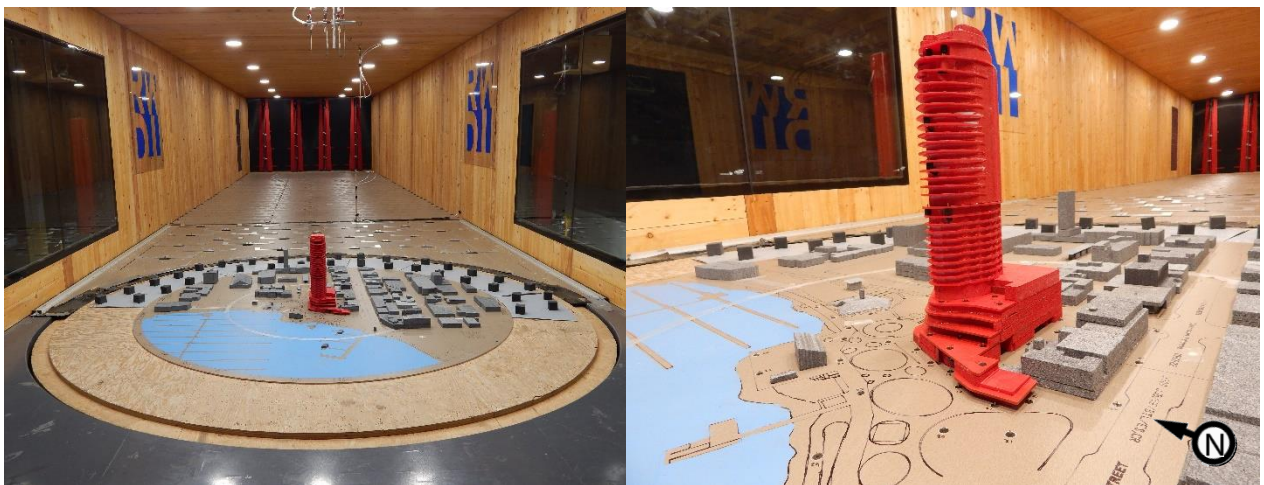
Image 2b: Wind tunnel study model - Proposed configuration
